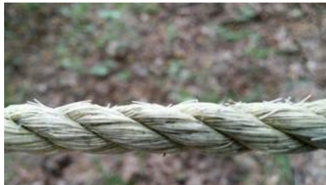
Picture of frayed guide ropes that have been replaced
